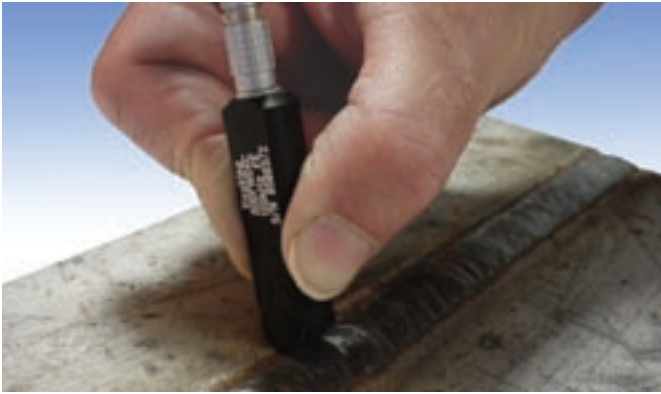
Weld inspection with a specially designed WeldScan probe.
