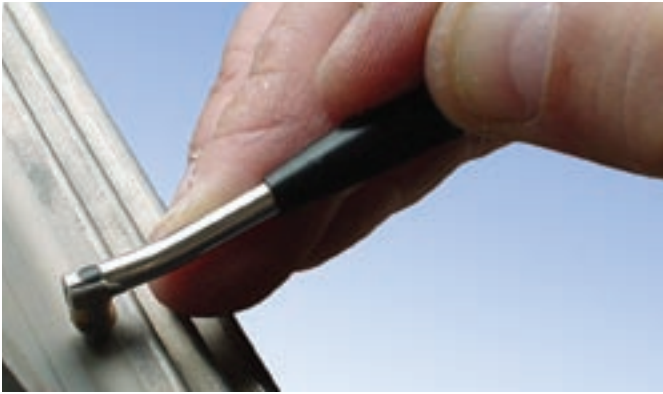
Surface inspection using an absolute pencil probe.
