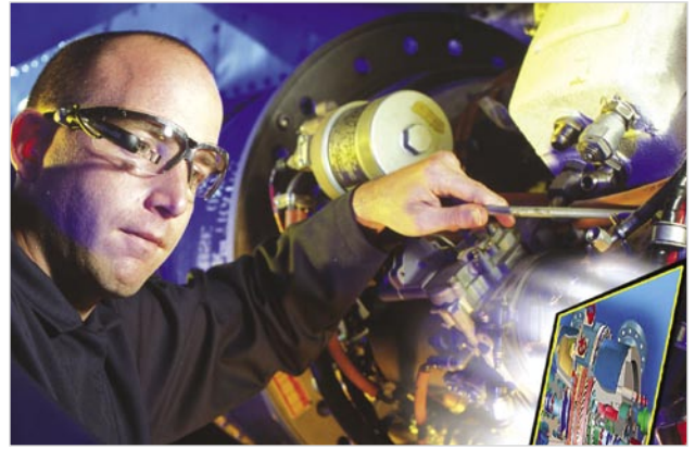
■ The MicroOptical CV-3 used in aircraft engine inspection
