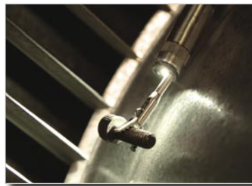
■ Bolt retrieval using 3 mm Alligator working tool
