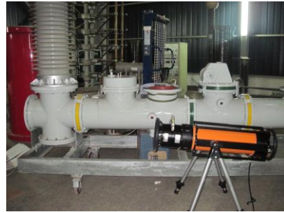
Fig. 5 X-ray machine and the imaging plate
