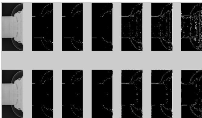
Fig. 11 the edge detection based on before and after wavelet de-noising of not fully closing position2
